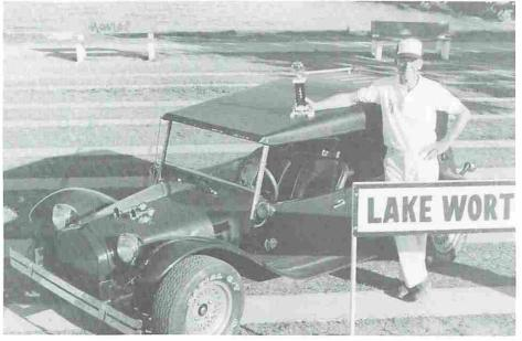
Bentley. It has a 4-cycle engine, no radiator, and gets 25 miles on a gallon of premium gasoline. This 4 passenger touring car has a fiberglass top, plastic and leather side flaps, radio, heater, and voltage regulator. The engine is air cooled, starts with a mini-battery and has 4 manual shifts. The car has a special two-toned horn and weighs 1875 pounds. It is valued at \$65,000.
