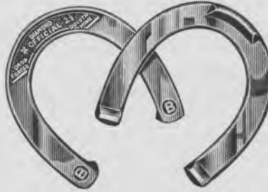
Curved Toe Calk Official Shoe. Made in weights 2 lbs. 5 ozs.; 2 lbs. 6 ozs.; 2 lbs. 7 ozs.; 2½ lbs. Diamond official pitching horseshoes are all drop forged from high grade steel, heat treated and drawn in oil. Will not chip or break.
