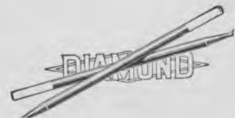
Official steel stakes. 10 inches above ground painted white aluminum; rest rust-resisting black. 30 inches overall.
